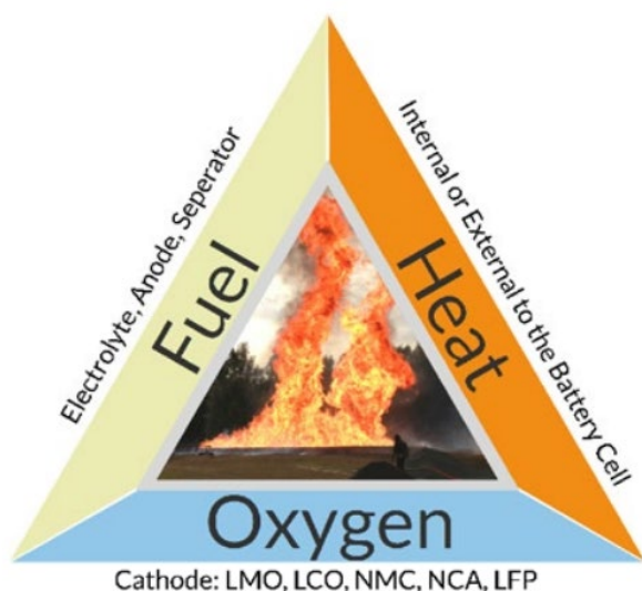
Figure 2: The fire triangle for Li-ion batteries [20]
