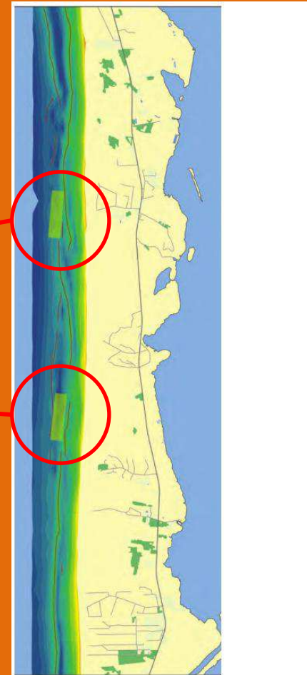
Fig. 4.1.1 2011 nourishment areas. Arrows indicate aim distribution of the nourished sand
