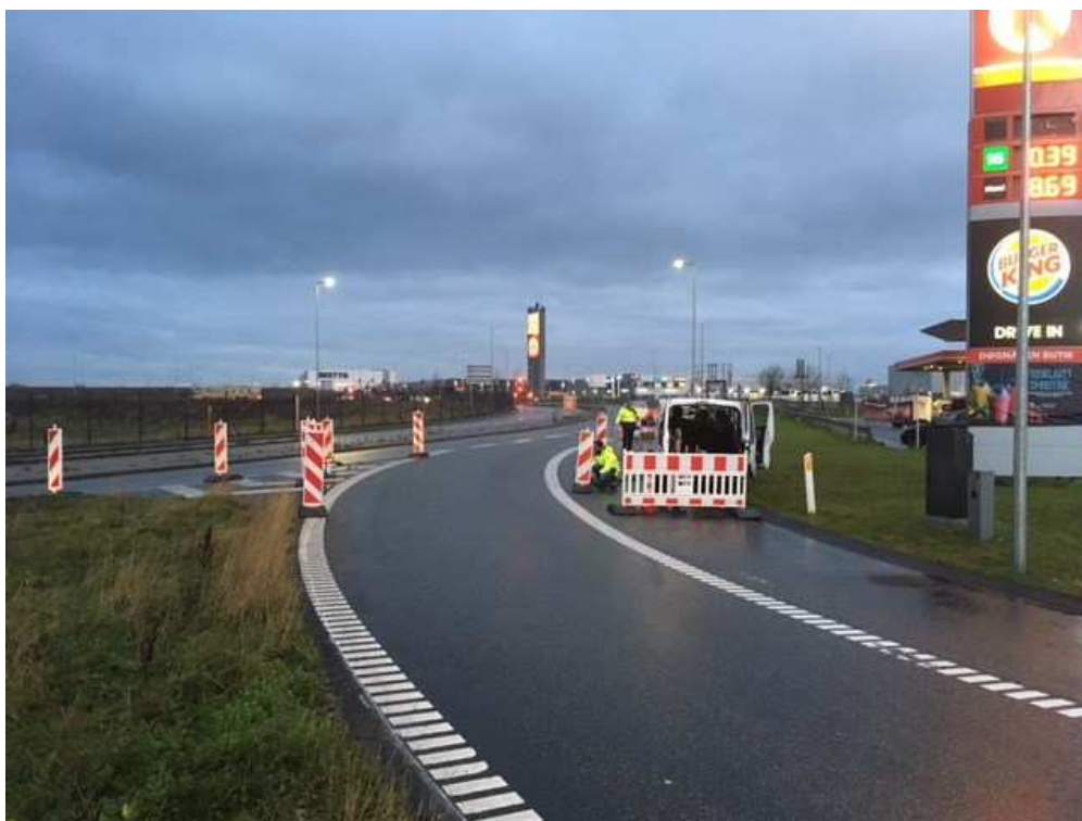
FIGURE 2.7. The measurement site at the Scandinavian Transport Centre in Køge. The van and the Spanish crew are seen on the right side of the curved road. The Source and receiver units are placed just behind the warning signs and the mirror units are placed opposite at the left side of the road. The construction site markings were setup especially for this measurement campaign.
