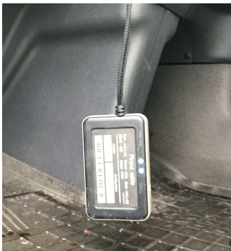
FIGURE 3.8. Picture of cheating device found in one of the heavy duty vehicle that was inspected by the Danish Police in Padborg.
