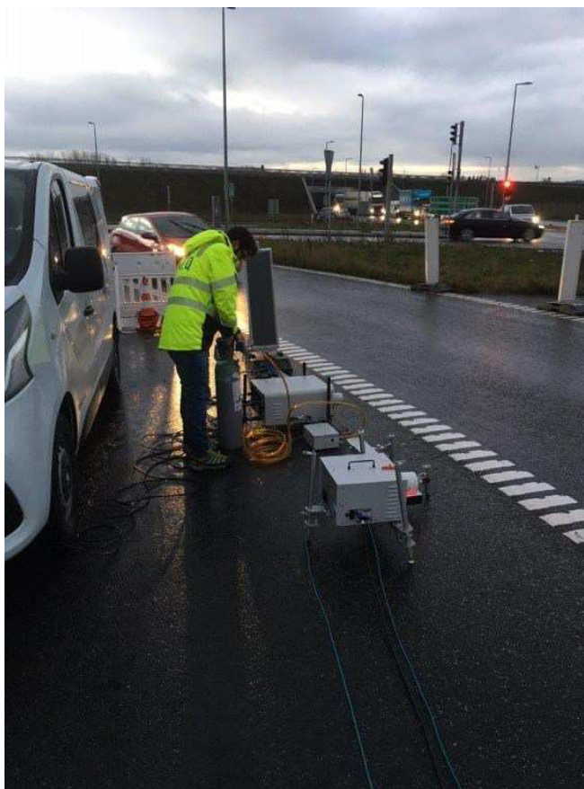
FIGURE 2.3. The remote sensing devices were calibrated several times during a day by use of certified calibration gasses.
