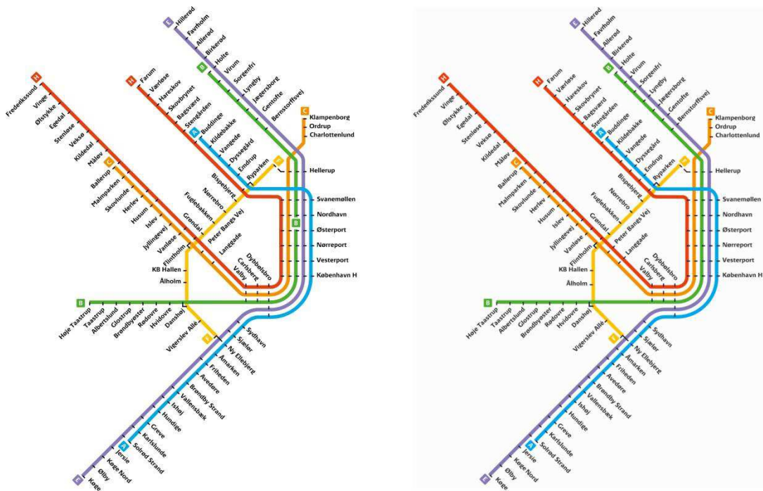
Figure 3: Flex 36 scenario. Stop pattern in peak periods (left). Stop pattern in non-peak periods (right)
