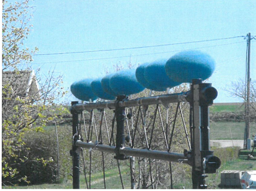
Figure 8: Microphone array at the receiver point.
