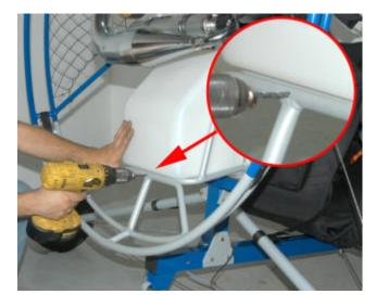
Assemble the two upper cage frames and insert the special lower cage frame.
