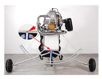
This terminate the engine mountig SETUP that is required ONLY for an eventally change of the engine model with different holes position.
