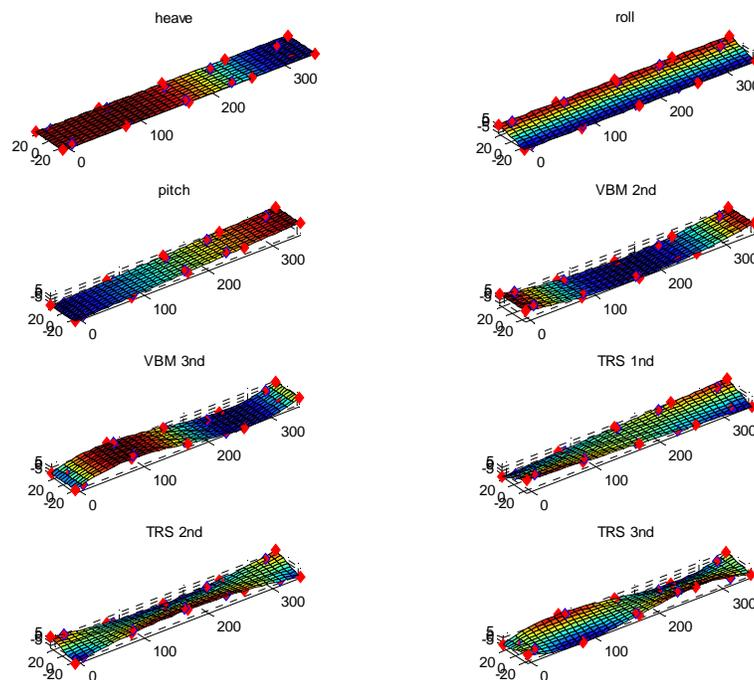
**Figure 10 Hull deformation parameterisations**
