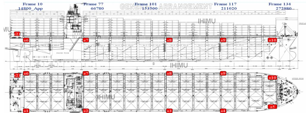
Figure 6 NYK Argus - Accelerometer sensor grid
