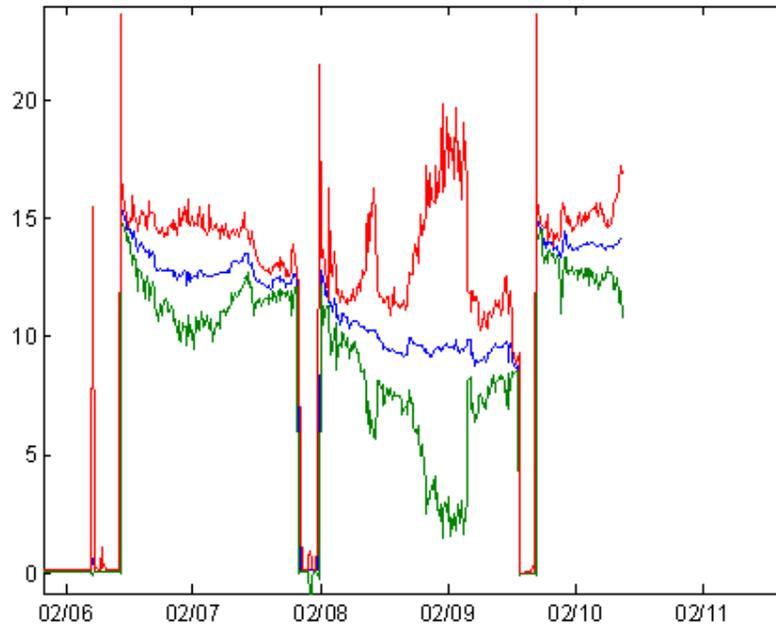
Figure 24 Typical web lashing force recordings [KN]
