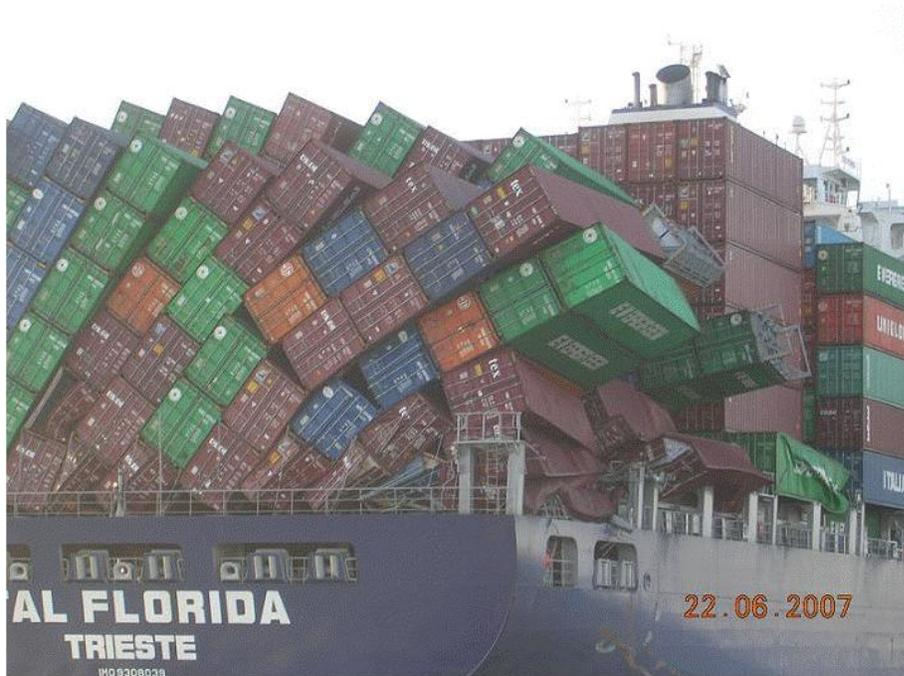
Figure 17 Incidents - Unexplained bay collapse / loaded containers
