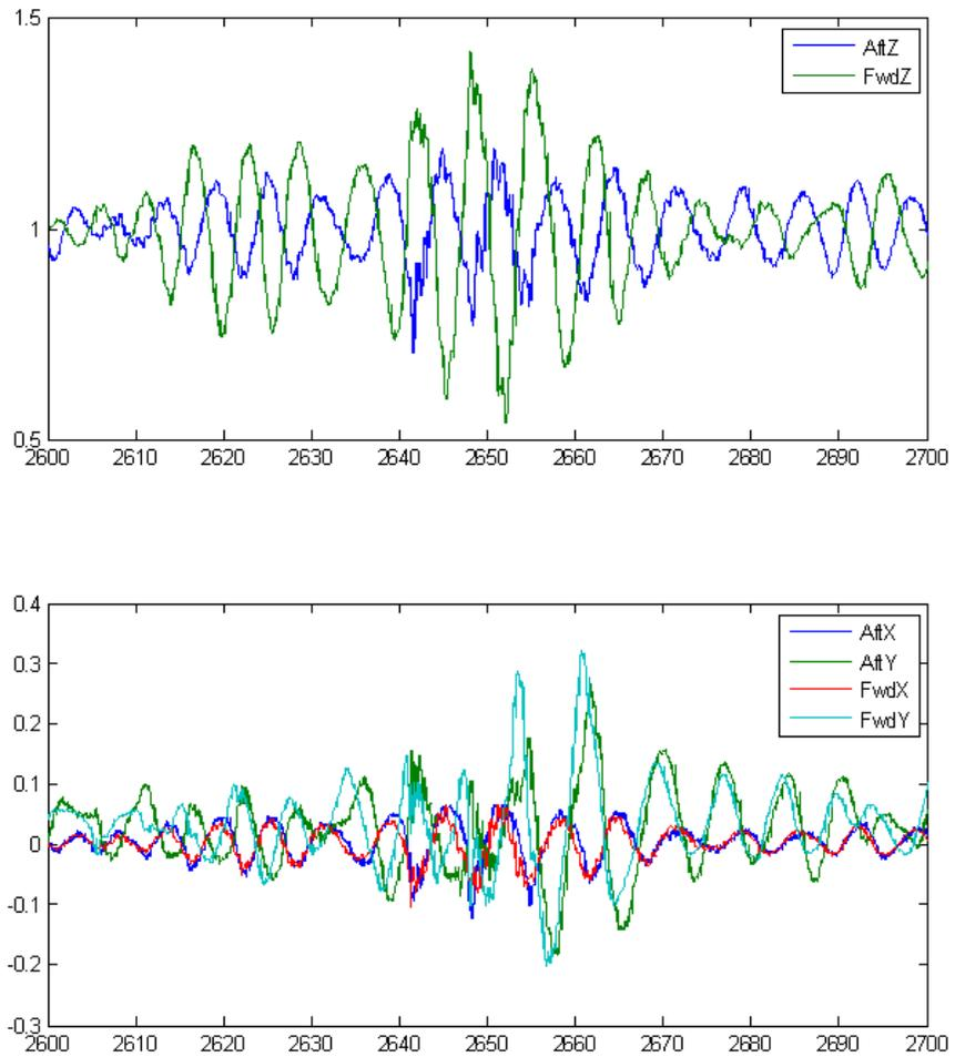
Figure 22 Measured g-loads in transit Schieborg
