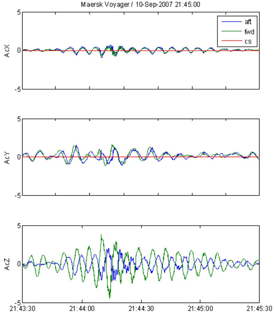
**Figure 23 Measured accelerations Maersk Voyager [m/s<sup>2</sup>]**
