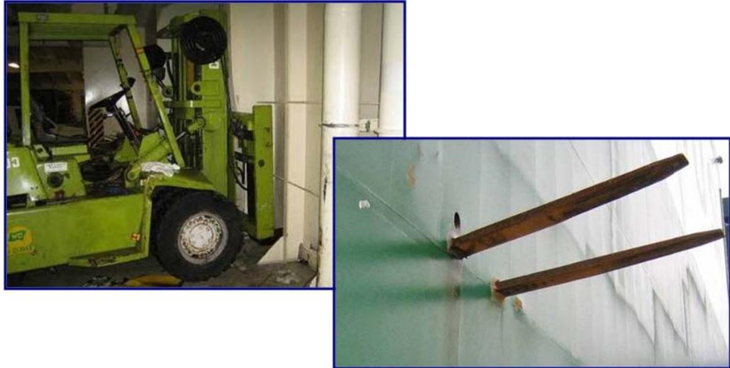
Figure 12 Incidents - Consequential damage by cargo shift
