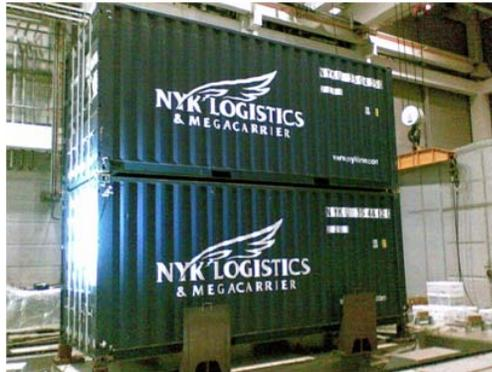
Figure 7 MCS - Full scale container tests 2 tiers
