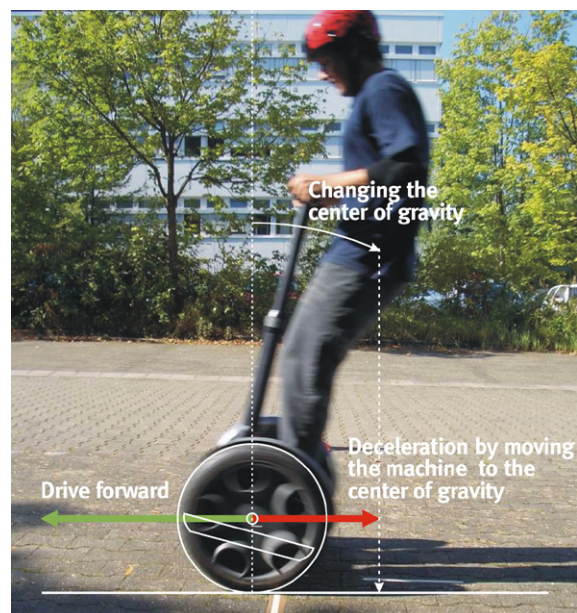
Figure 20: demonstration of the process of braking
