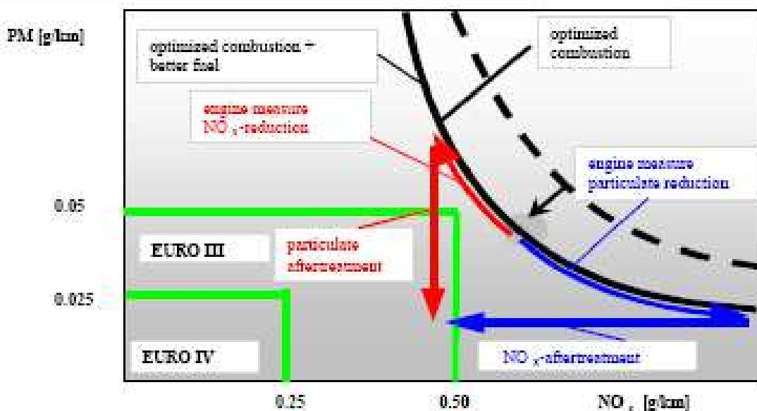
*NO<sub>x</sub>/PM trade-off-curve for passenger cars. Emission values refer to NEDC- cycle. Similar principle is valid for heavy-duty trucks.*
