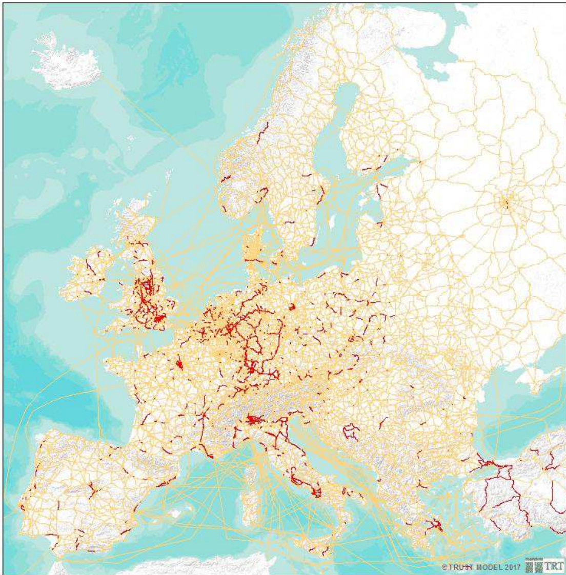
Figure 4-13: Congested links in TRUST 2030 network (Daily load/capacity ratio \geq 0.5 )
