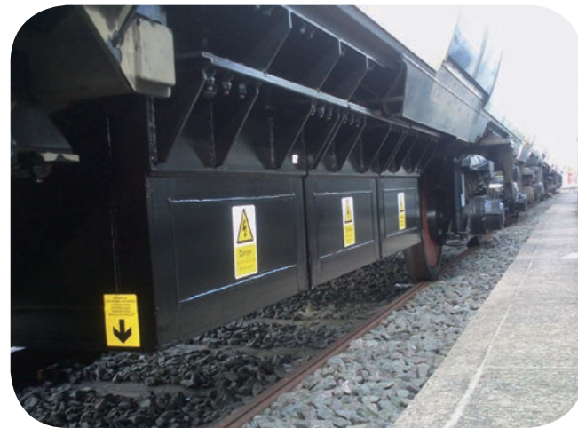
Mounting of three battery rafts on the ELECTROSTAR train
