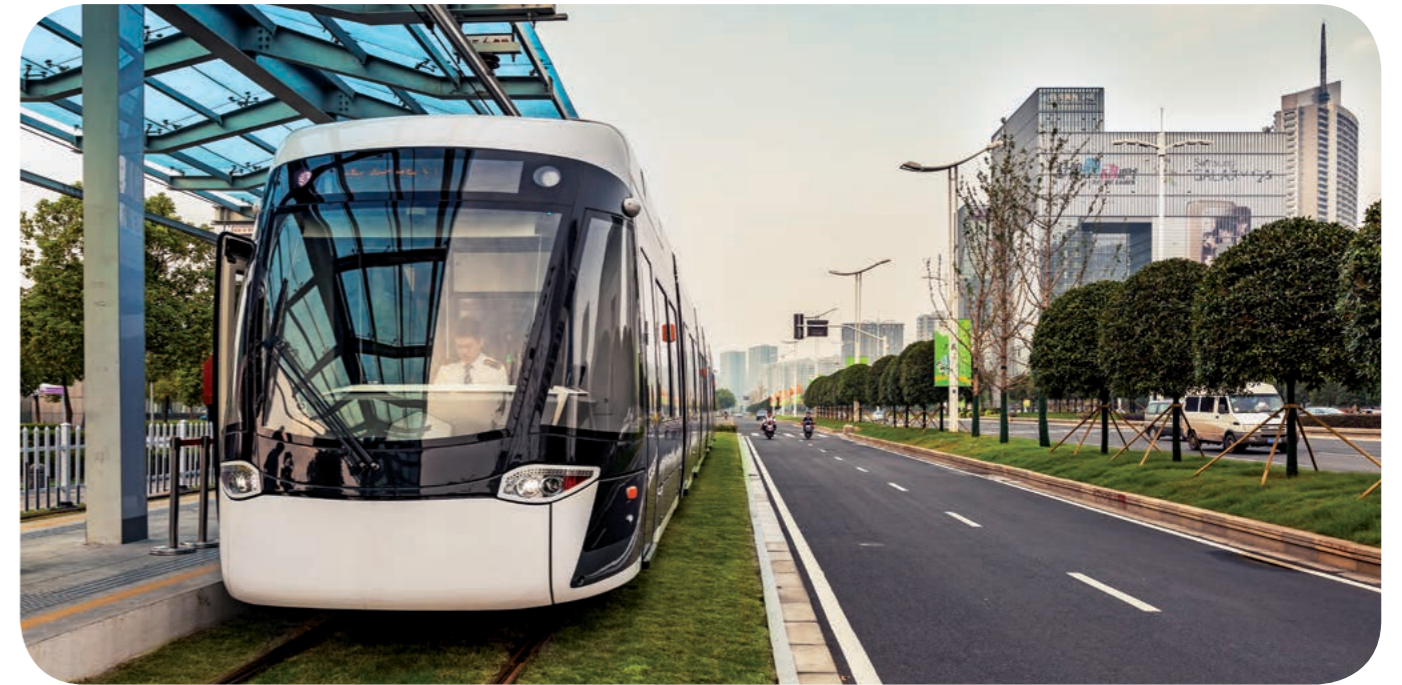
The catenary-free operation tram for Nanjing is based on BOMBARDIER* FLEXITY* 2 tram technology, equipped with the PRIMOVE lithium-ion traction battery systems for trams, MITRAC* propulsion equipment and FLEXX* Urban 3000 bogies.
