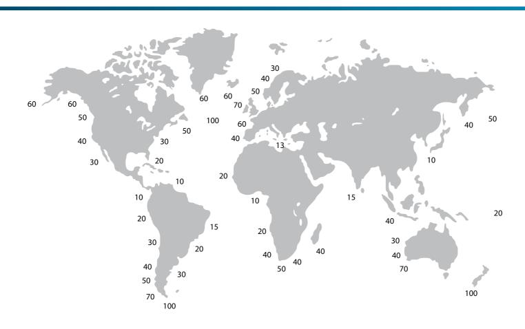
Note: the numbers on the map express the wave energy potential at the specific site – the higher the number, the greater the potential (kW/m wavefront)
