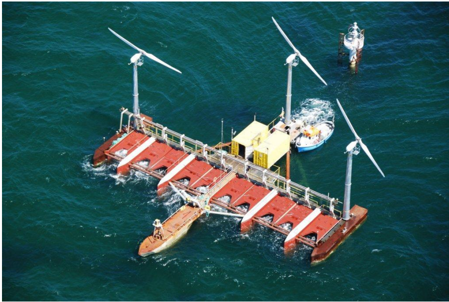
Figure 29 Floating Power Plant [w39]
