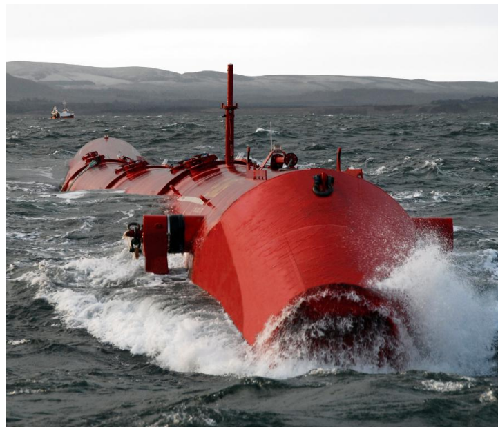
Figure 2 Pelamis wave energy converter off the coast of the Orkney Islands [w2]
