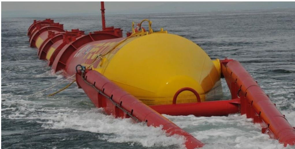
Figure 23 Pelamis 2 During towing towards EMEC test site.
