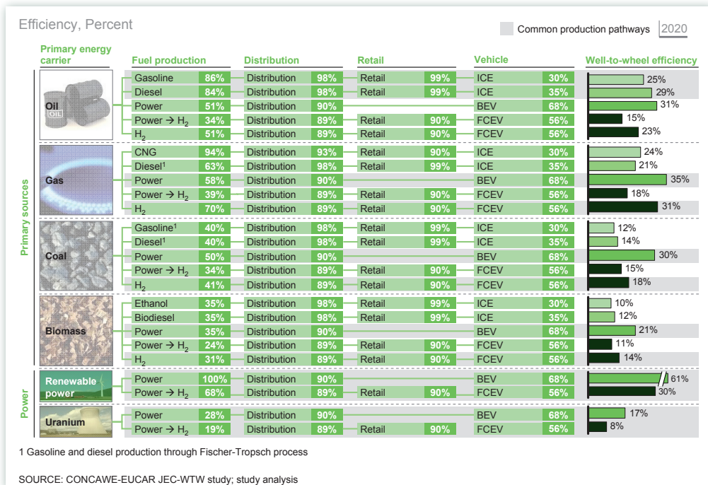
Exhibit 43: FCEV well-to-wheel efficiency is competitive with ICE, with a flexible use of feedstocks, while BEV remains the most efficient power-train
