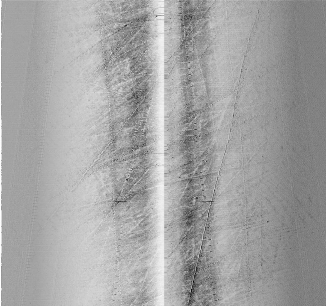
Figure 3.2: Side-scan image of tracks from trawl boards in the area north of Bornholm.
