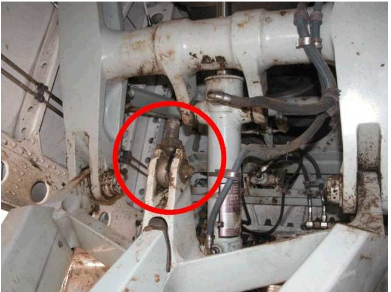
Figure 1: View of separated rod end.
